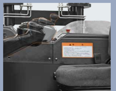
The steering wheel is extensible, so the operator can choose the best driving position
