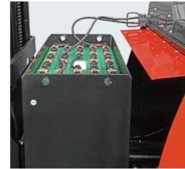
Battery can be removed forward, easy for maintenance
